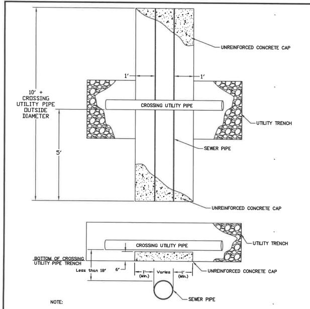
UNREINFORCED CONCRETE CAP IS TO BE SIZED BASED ON THE FOLLOWING DIMENSIONS:
